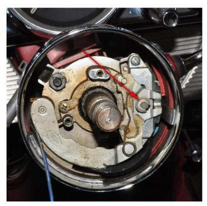
Pull the canceller lever out. Now the nut at 5 o'clock is visible. Don't remove it yet though, and actually, leave
