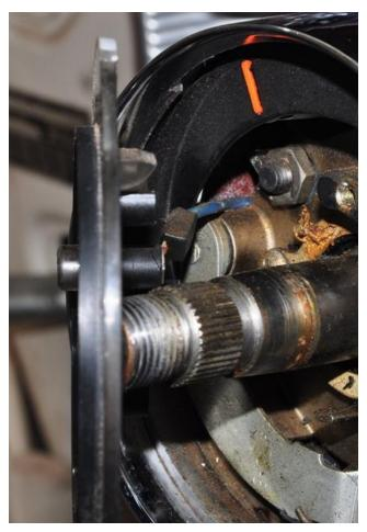
for the blue/yellow stripe wire at the base of the steering column. While pushing on it a bit to give it slack, I gently pulled the wire until I had enough slack to work.
