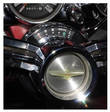
Now, once you get that spring and horseshoe back on, you're home-free with a nice tight shifter. It's actually in park now and feels like it will stay there. The indicator plate is adjustable, so place the shifter in park, line up the plate, and tighten the screws before replacing the steering wheel.
