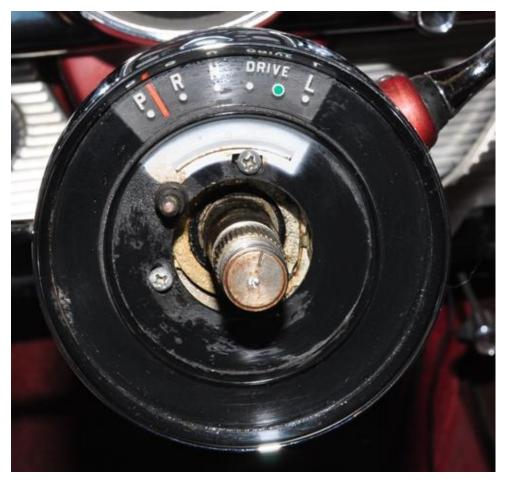
Pull the horn contact out and the two drive indicator plate screws and set them aside with all your other parts. You'll have a lot of small stuff to keep track of. I used a magnetic tray.
