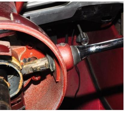
To remove the shifter, rotate it 90 degrees down to free it from the rear pressure pin. It then pulls out easily. Just reverse the process when installing the new shifter. If the rubber binds up during installation, smear a small dab
