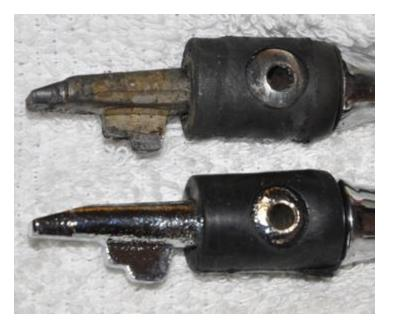
Here is my problem. The edge has chamfered on the shift lever. This thing was a time-bomb, ready to fall into reverse.
