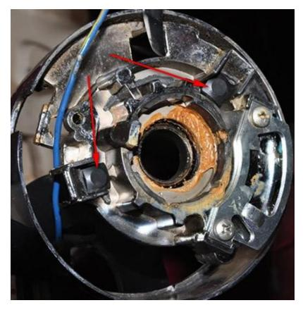
During reassembly, put the retaining bolts in the back, and in the front, thread the nuts on a couple turns. Then, using a thumb on each nut, push them outward until the whole assembly snaps back into place and the square bolt heads are engaged into the outside of the slots shown..
