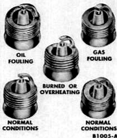
FIG. 7—Spark Plug Inspection
