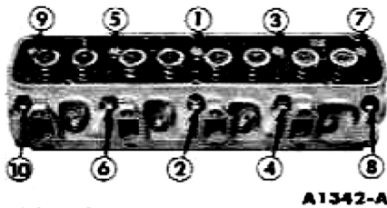
FIG. 46—Cylinder Head Bolt Tightening Sequence
