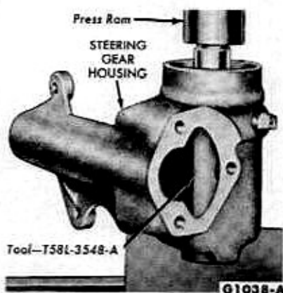
FIG. 9—Steering Shaft Lower Bearing Cup Installation
