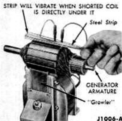
FIG. 6—Growler Test for Shorted Armature
