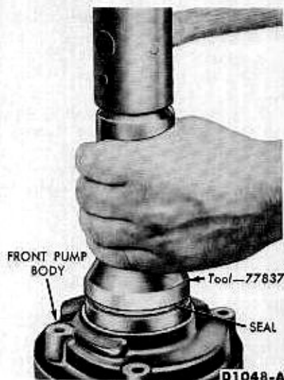
FIG. 17—Front Seal Installation
