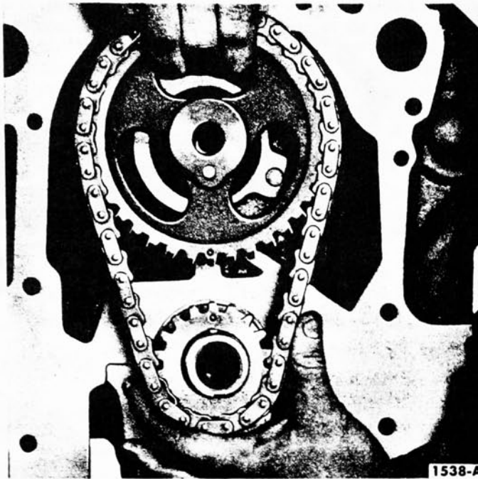
FIG. 21—Timing Chain Removal or Installation
