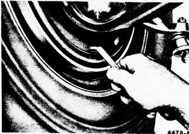
FIG. 3—Brake Shoe Adjustment
