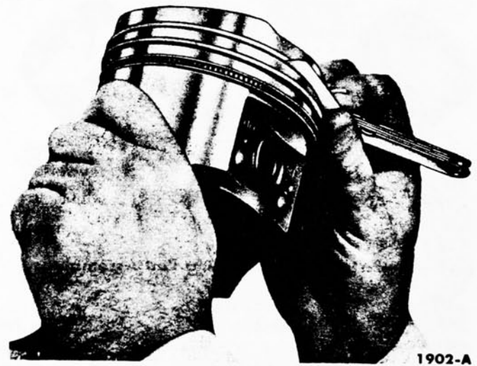
FIG. 30—Ring Side Clearance
