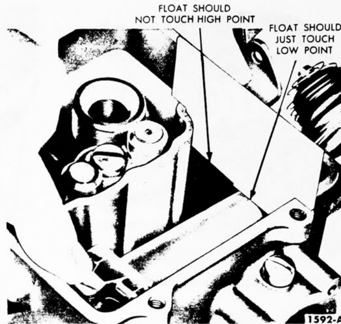
FIG. 25—Float Adjustment
