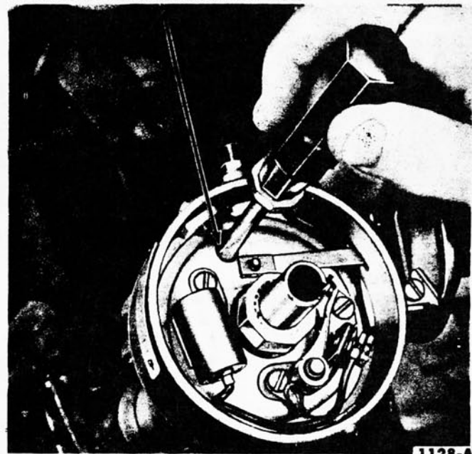
FIG. 12—Centrifugal Advance Adjustment
