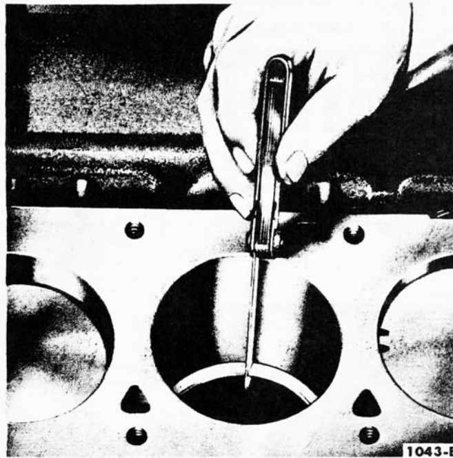
FIG. 20—Piston Ring Gap—Typical
