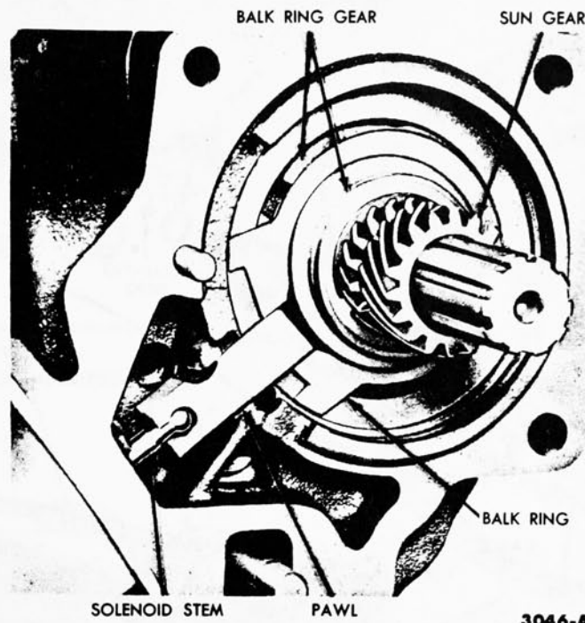
FIG. 9—Pawl Engaged in Balk Ring Gear
