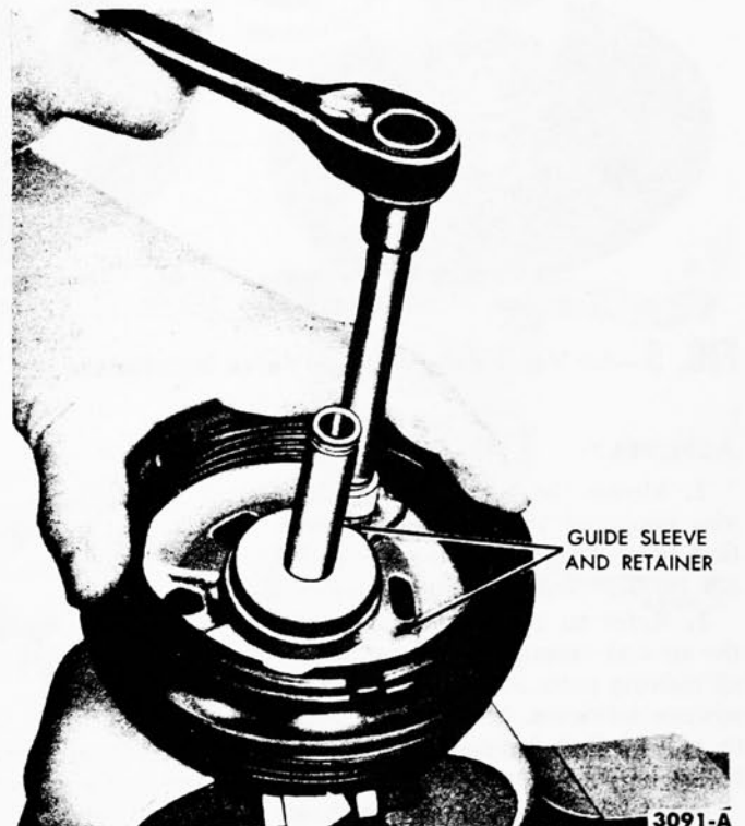
FIG. 8—Guide Sleeve and Retainer Removal
