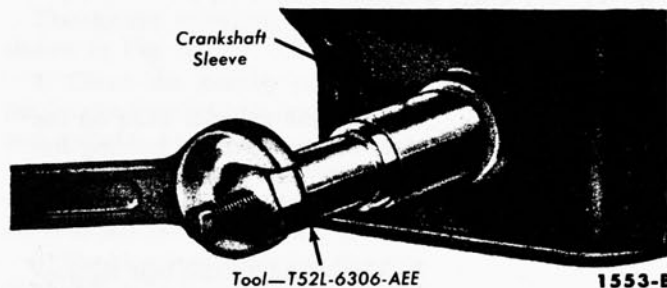
FIG. 48—Crankshaft Sleeve Installation
