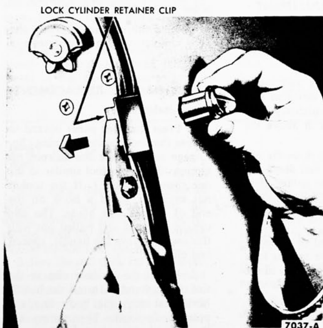
FIG. 3—Lock Cylinder Removal
