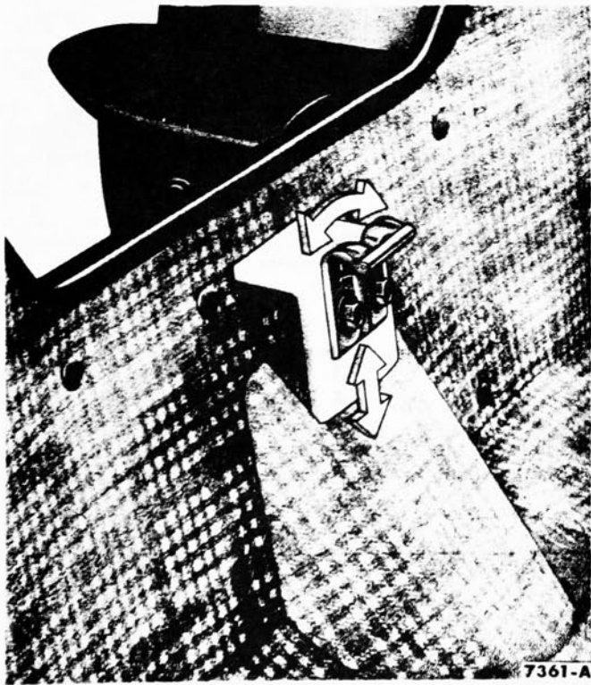
FIG. 12—Deck Lid Striker Plate Adjustment
