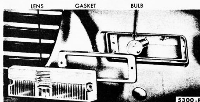
FIG. 8—Parking Light Disassembled
