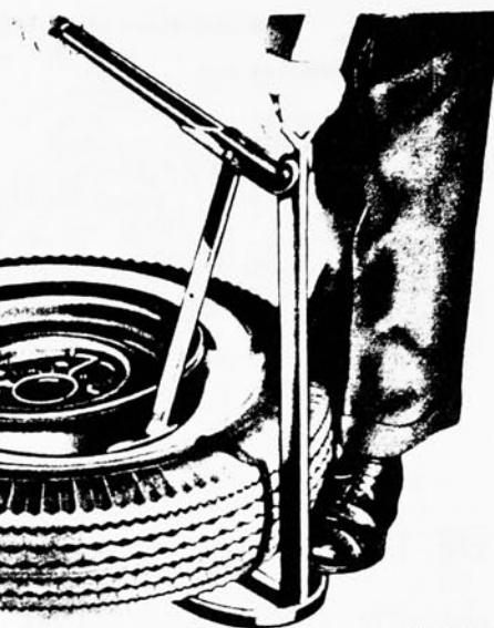
FIG. 4—Bead Loosening Tool
