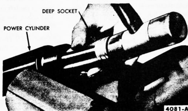
FIG. 20—Power Cylinder Seal Installation
