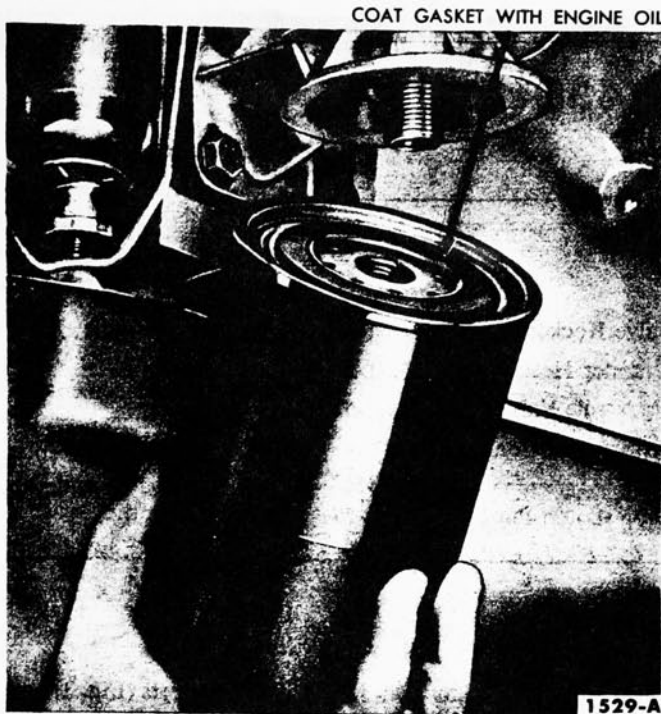
FIG. 58—Oil Filter Replacement
