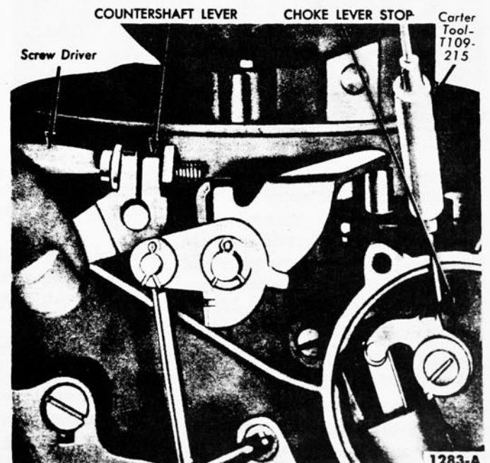
FIG. 50—Choke and Countershaft Linkage Adjustment
