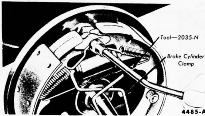
FIG. 10—Retracting Spring Removal
