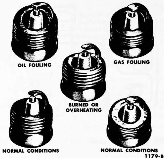
FIG. 7—Spark Plug Inspection
