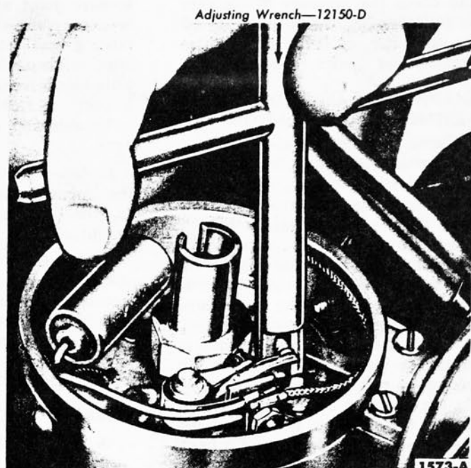
FIG. 16—Aligning Breaker Points
