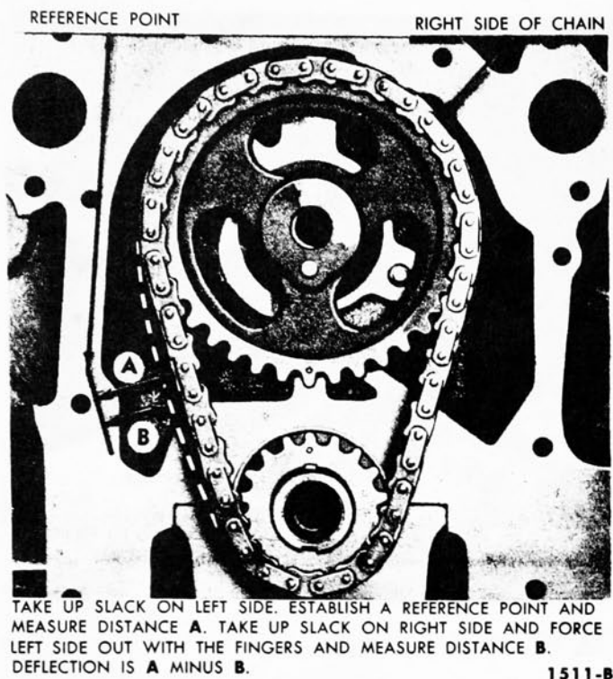
FIG. 44—Timing Chain Deflection
