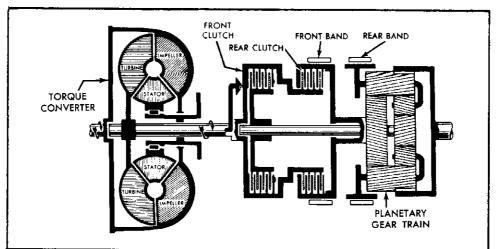
The drive components of the transmission consist basically of a torque converter, clutches, bands and a planetary gear train. Automatic control of the mechanical elements is provided by a hydraulic system. Detailed picturization of the entire transmission is shown on page 2.
