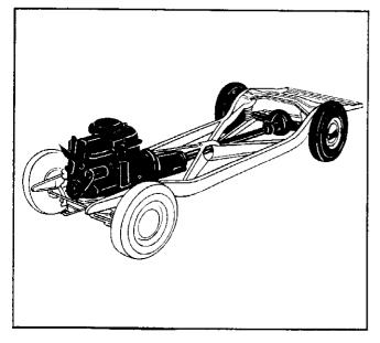
The function of this transmission is the same as that of any other transmission to -- provide suitable gear ratios between the engine and the rear wheels to meet all driving conditions.
